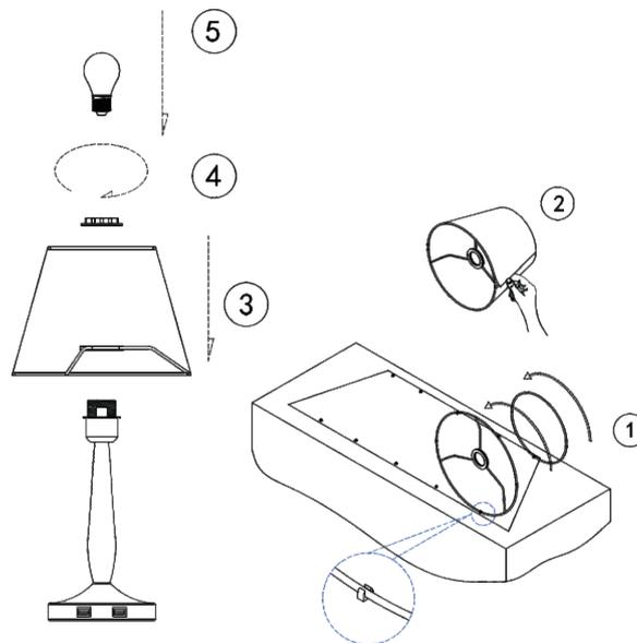
①② Place the two rollers on the lampshade in the same direction as shown in the figure, and press them on the plastic buckle to make them completely coincide, pay attention to the inner installation of the roller protruding part towards the lampshade.
