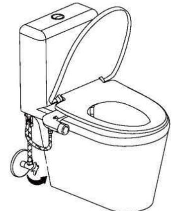
Adjust the knob according to the picture showing, turn on the angle valve, and then check if any leaking happening in each connector.
