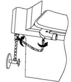
To assemble the braided hose to the water inlet end of bidet and turn tight.
