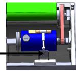
Fig. 6, adjusting bolt -
